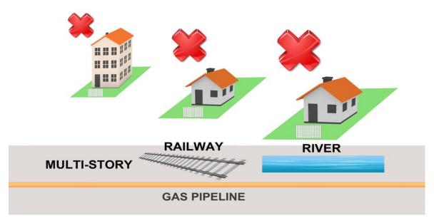
The three examples illustrated above require an engineering site visit to determine if the property is connectable and the costs associated with the service and meter installation.
