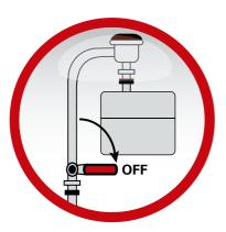
Turn the emergency control valve to the 'off' position. It is off when the lever is at a right angle to the pipe.
