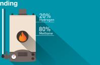
Modern gas boilers and appliances can accommodate a methane/Hydrogen blend of up to 20% Hydrogen. Consumers should anticipate Hydrogen to be first blended into the NI Gas Network from the middle of this decade.
